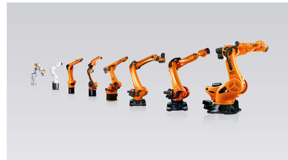
Figure 1. Examples of six-axis, articulated-arm robot.
