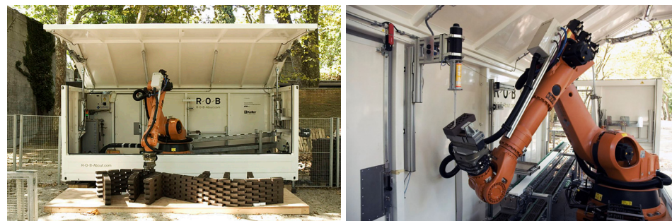
Figure 19. ( Top) Conceptual design ROB Unit; (bottom left) ROB Unit assembling a segment of the Structural Oscillation installations; (bottom right) ROB Unit set-up.
