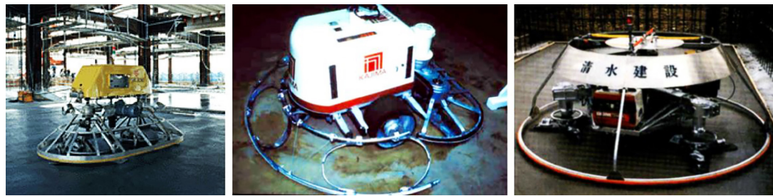
Figure 14. Concrete finishing robots: (left) SurfRobo by Takenaka Corporation; (middle) Mark II, also known as Kote-Kirg by Kajima Corporation; (right) FLATKN by Shimizu Corporation.
