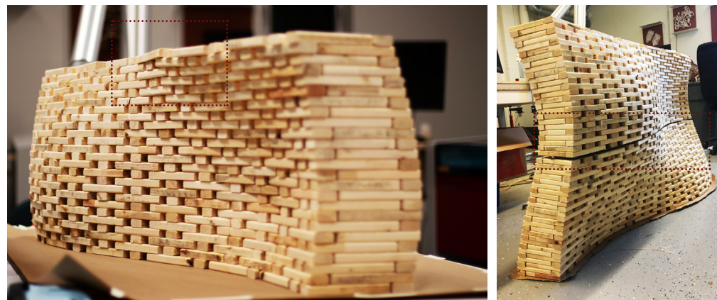
Figure 65. The accumulated error due to the dimensional tolerances and imprecision of components: (left) the accumulated error of fabricated piece; (right) gap variances in the assembly of two sections due to the accumulated error.
