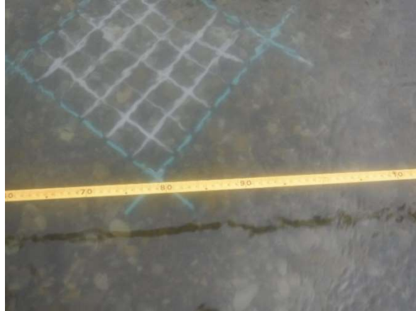
Figure 2.5. Sampling grid for bed roughness measurements
