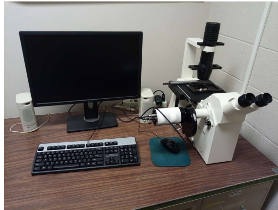
Figure 2.4. Floc imagery equipment including Wild Leitz inverted microscope equipped with a Sony XC75 CCD camera
