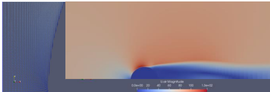
Fig. 26: Vector plot near stagnation point and velocity magnitude field over the cylinder, in m/s.
