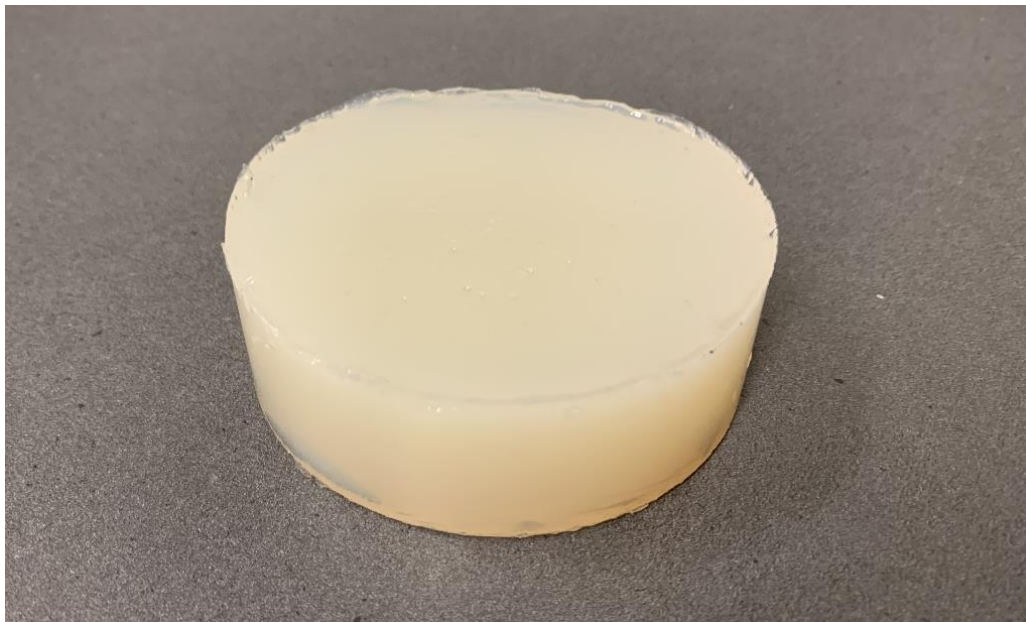
Figure 4-6 A low-absorption phantom after solidification.
