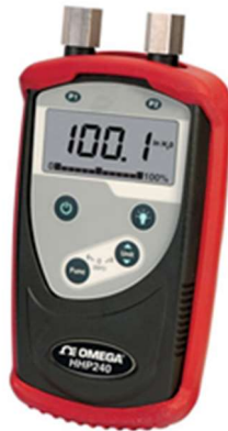
Figure A-4. Digital manometer (sensitive pressure gauge) used to calibrate the methane pressure.
