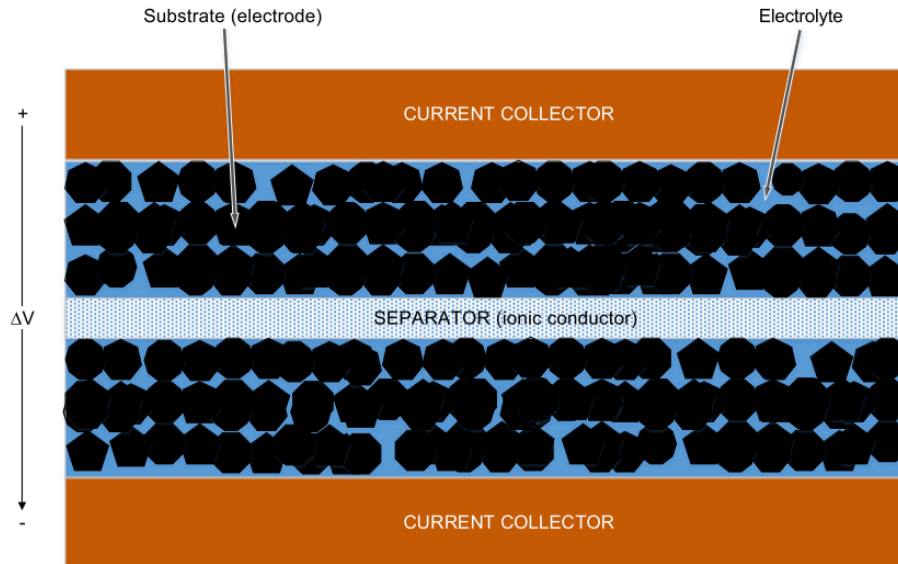
Figure 2: Schematic diagram showing components of a Symmetric Supercapacitor (Reproduced from reference [29]).
