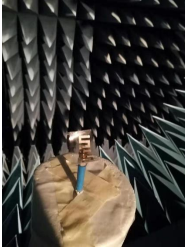
Figure. 4.9. Optical image of LPC antennas being tested in the anechoic chamber.
