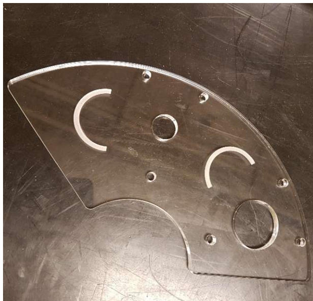
Fig. 3-13. Prototype of a sample holder for a smaller sample in permeability measurements.
