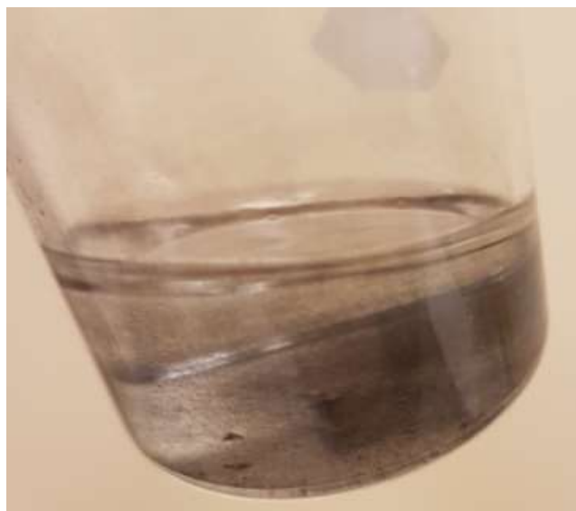
Fig. 4-5. Carbon particles present in octane after the preparation of the 0% PTFE sample for the Method of Standard Porosimetry.
