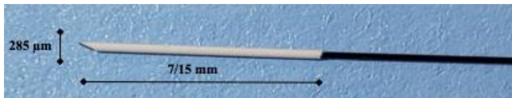
Figure 6.2 Biocompatible solid phase microextraction (Bio-SPME) probe
