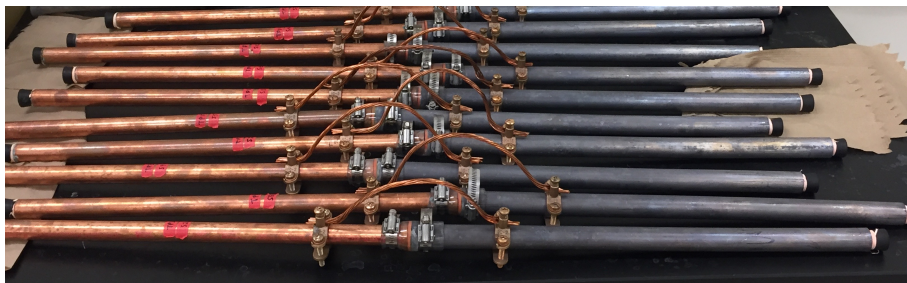
Figure 3.2 Lead and copper test pieces utilized in the experiment. The lead and copper pipes were attached using flexible PVC tubing and separated using a rubber hose washer. The galvanic connection was provided through the use of bronze ground clamps and copper ground wire.
