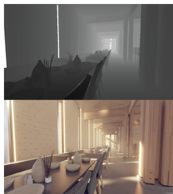
Figure 31: A Depth Buffer (Mapped to Greyscale), and its Corresponding Rendered Scene.
