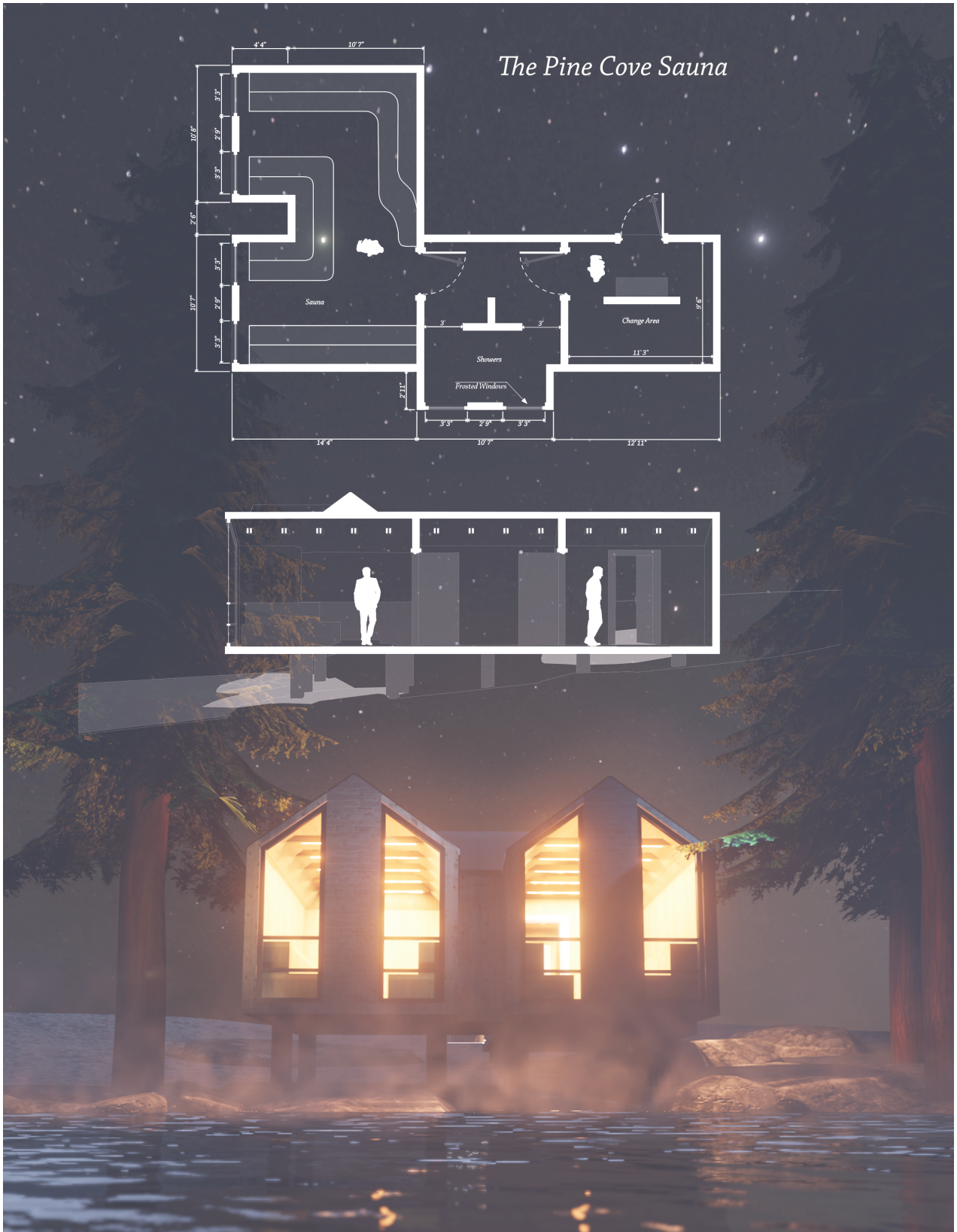
Figure 84: Pine Cove Sauna - Conceptual Render Blender Eevee render overlaid with a MeasureIt-ARCH plan and section.
