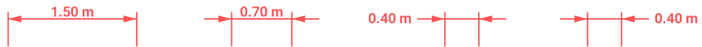
Figure 75: MeasureIt-ARCH Dimension Text Placement. A dimension's text and termination arrows automatically adjust their placement to avoid overlapping.
