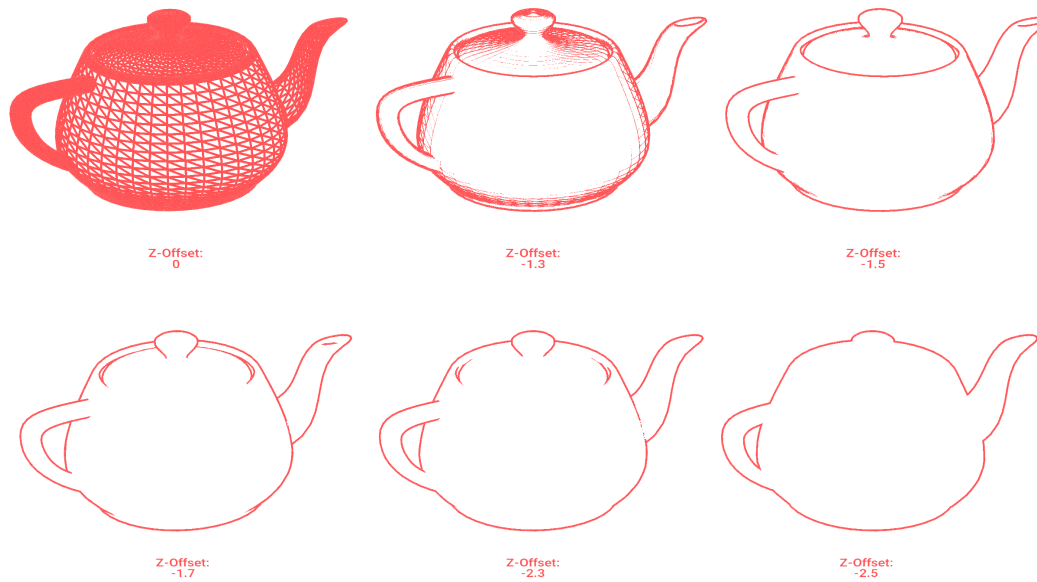
Figure 57: MeasureIt-ARCH Silhouette Lines A progression showing how the display of Variable Silhouette lines change as the Z-Offset value is adjusted
