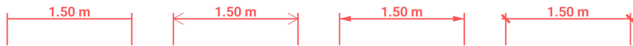
Figure 62: MeasureIt-ARCH Dimension Terminations. From Left to Right: None, Arrow, Filled Arrow, Dashed
