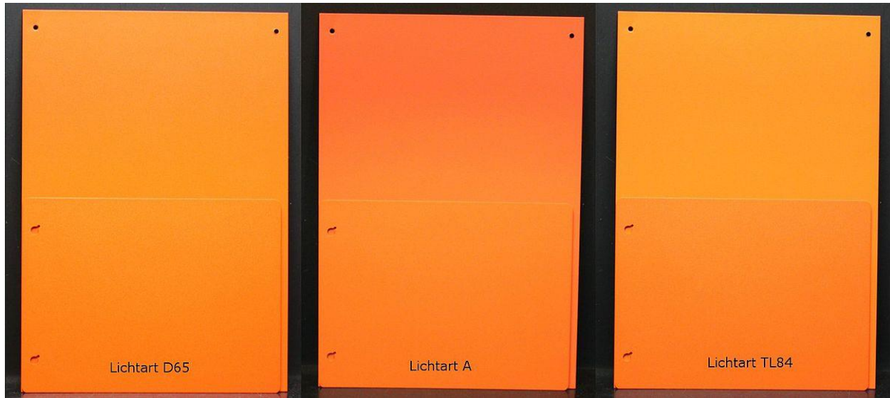
Figure 1.4. An example of metamerism. Two panels are shown under three different light sources. Left: daylight with a CCT of 6500 K, middle: an incandescent lamp with a CCT of 2856 K, right: a fluorescent tube light with a CCT of 4100 K. 17
