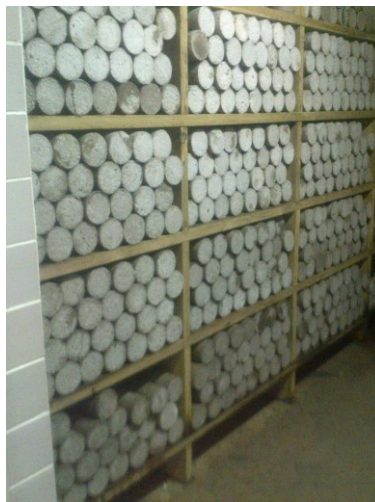
Figure 3-15: 400 cylinders in the humidity chamber
