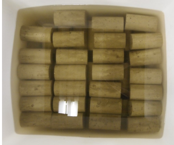
Figure 3-16: 80 cylinders submerged in the de-icing solution
