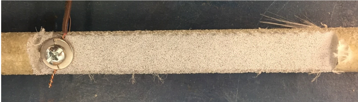
Figure 3-19: Digital Image Correlation sample specimen
