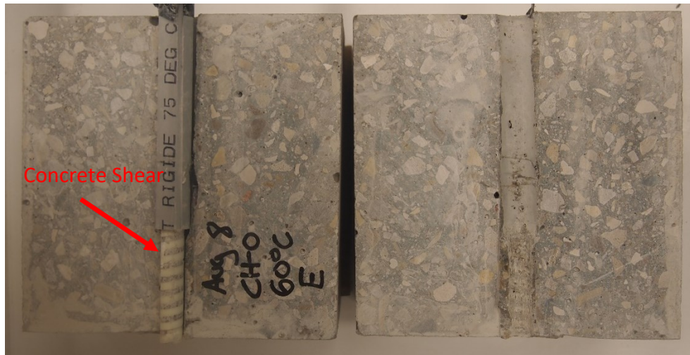
Figure 4-10: Autopsy of bond test specimen containing 12 mm Schöck – Combar
