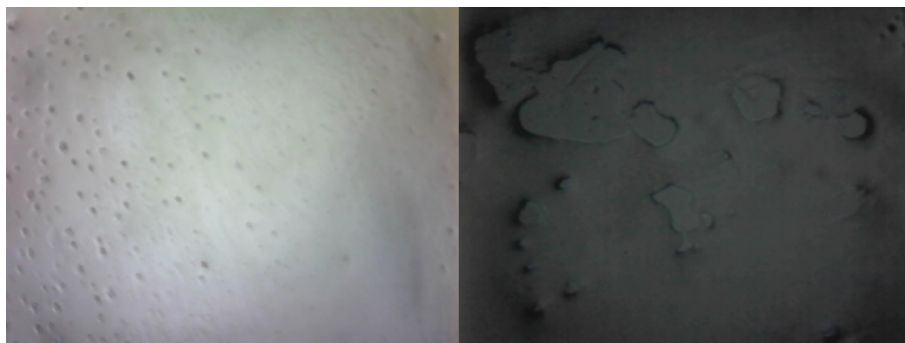
Figure A.22: Polarized optical microscope images of 8-CB mixture in 0.6 T environment (left) and 0.9 T environment (right). Mild imperfections can be seen on the left as dots. Darker image on the right arises from a rotated stage to spot any imperfections; none were spotted
