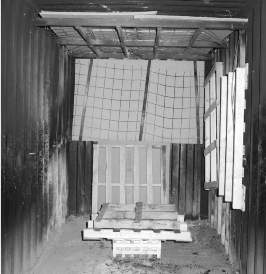
Figure 30: Mesh reinforcement for fibreboard
