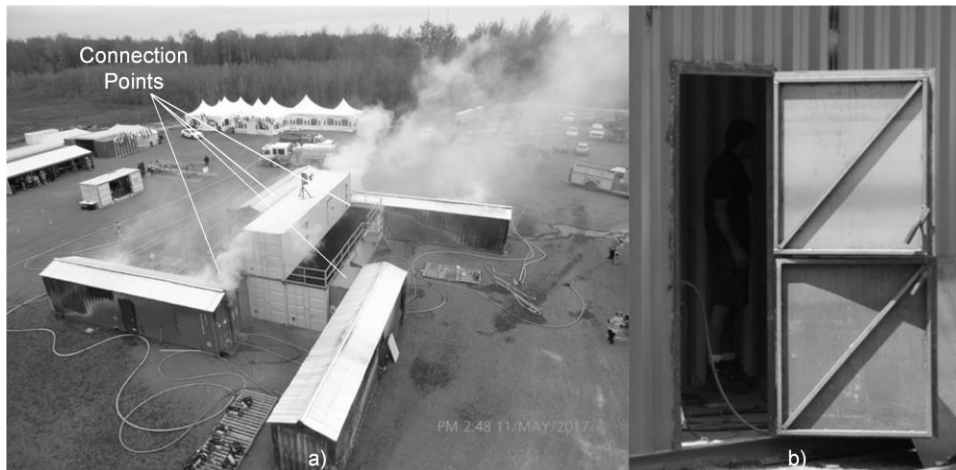
Figure 34: Side door: a) used to connect to larger structures; and, b) details
