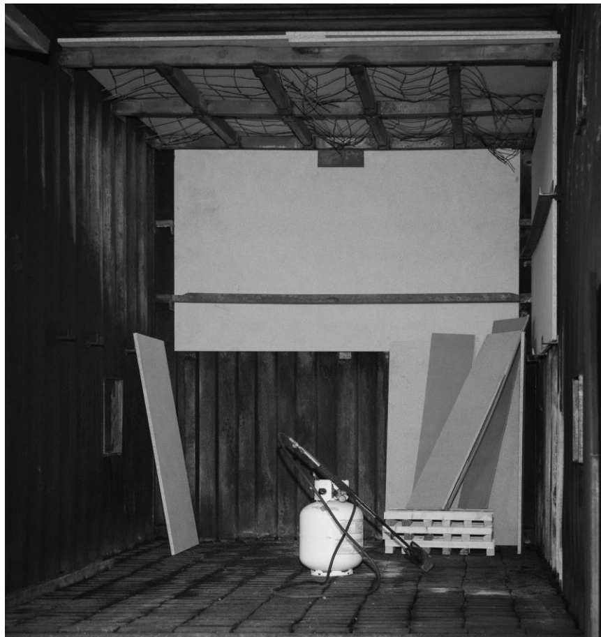
Figure 31: Final fuel support design for OFS training
