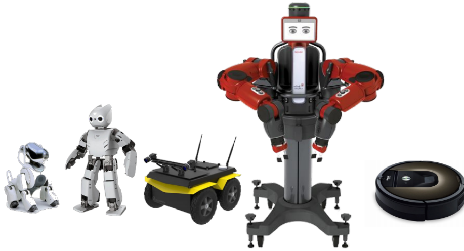
Figure 4.1: From left to right the robots pictured are Aibo (Sony) [Son19], DARWiN-OP (Robotis) [the19], Jackal (Clearpath Robotics) [Cle19], Baxter (ReThink Robotics) [Ret19], and Roomba (iRobot) [Per19].
