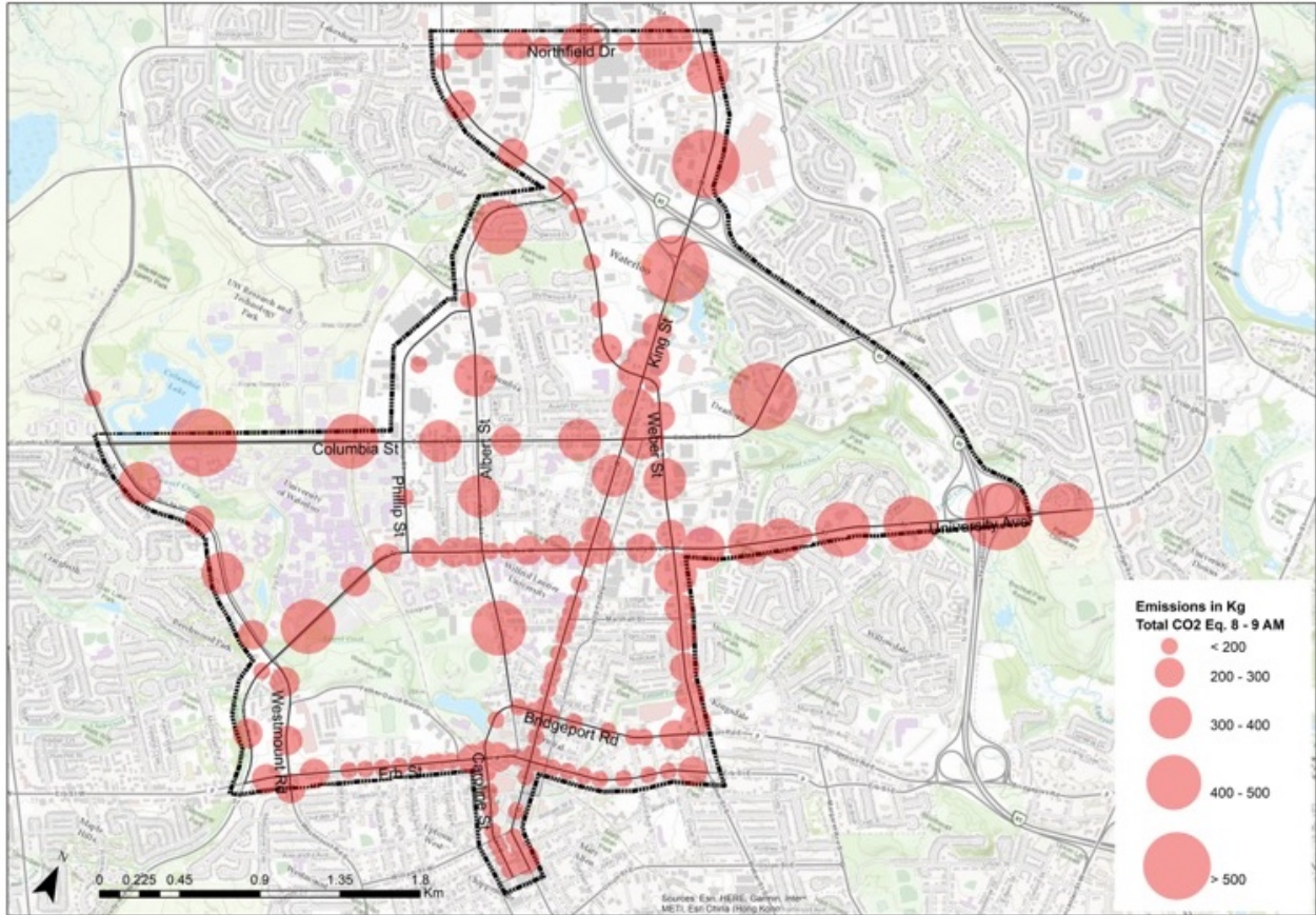
Figure 4-6: Road Segment wise Emissions (CO 2 Eq.) for the Peak Hour (8am to 9am)
