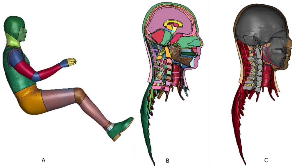
Figure 2-30: A) GHBMC 50 th percentile male full human body model B) GHBMC 50 th percentile male full detailed head C) GHBMC 50 th percentile male simplified head
