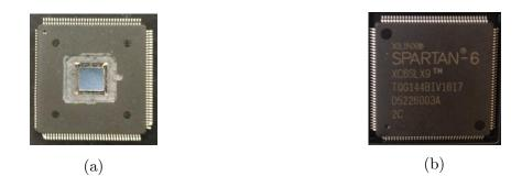
Figure 5.10: (a) Backside of the decapsulated Spartan-6 FPGA and (b) its unaltered frontside.
