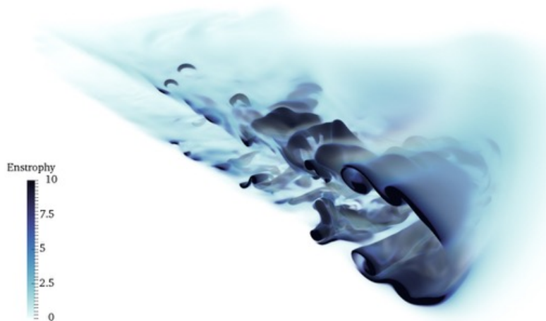
Figure 3.1: The rotation modified mode 2 wave discussed in [9]. The enstrophy field, which indicates energy dissipation, is shown. See text for details.
