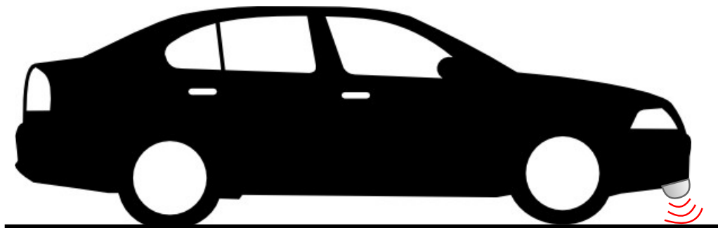
Figure 1.1: VIVA enables cars to sense the road condition using mmWave signals. VIVA’s sensor can be installed to the front (as shown here) or the rear side of the car.
