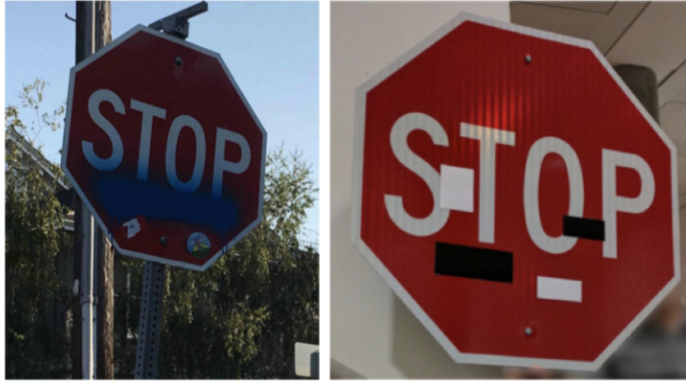
Figure 2.1: The left image shows a traffic sign with real graffiti on it, and the right image shows an adversarial Stop sign created in a similar fashion to the real one on the left. While most humans might ignore this perturbation, the right sign can fool the Sign detection system of an autonomous vehicle with a high probability [63]. Image from [63].
