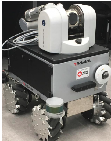
Figure 3.5: The omni-directional mobile robot used for validating the monocular VO algorithm with the proposed pipeline.
