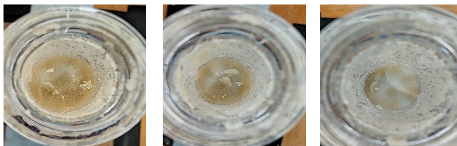
Figure B 4: Sigma Aldrich glass bead wet packed column, showing the column containing NPs before X-ray CT scanning (left) and the column showing obvious NP fingering during column dissection.
