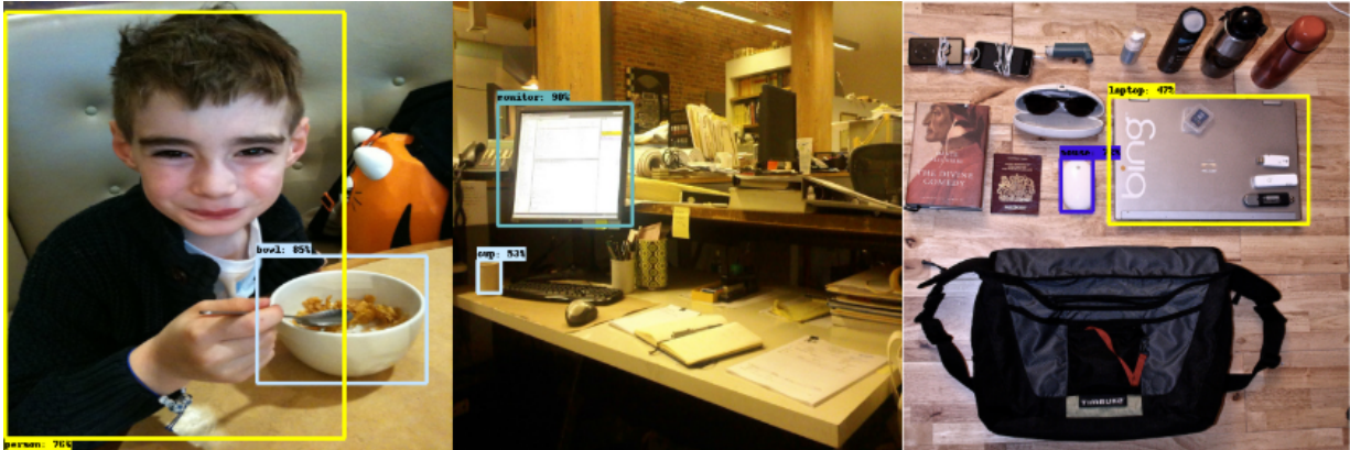
Figure 4.4: Sample detection results on MSCOCO-OLIV using MobileNetV2-SSD-1.13_224. All objects in Table 4.2 could be detected, however, left) the spoon is not able to be detected, middle) the book and small objects like the mouse are missed, right) even though the handbag is the largest object, it is not detected.
