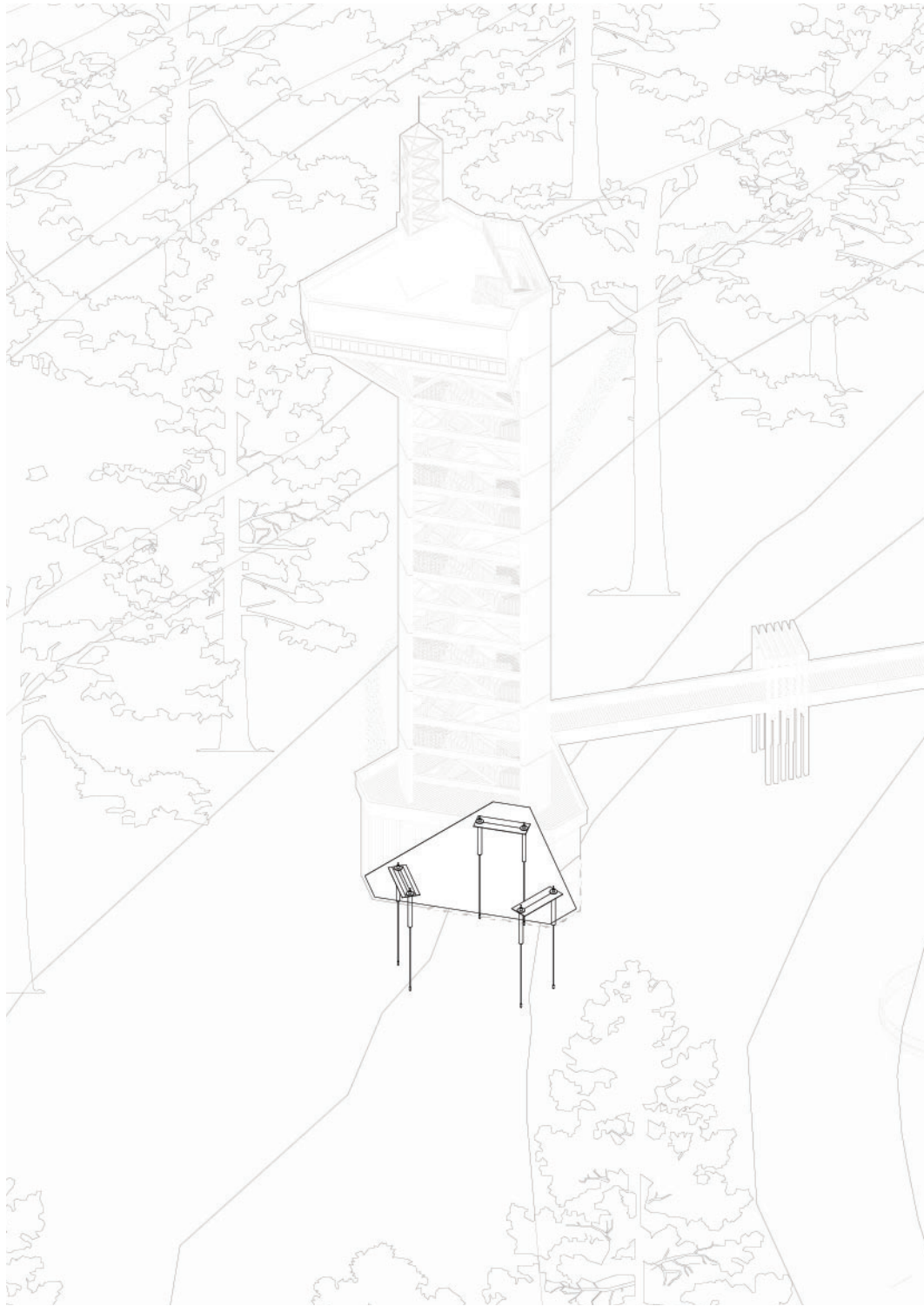
Figure 5.26 Structural Diagram: Rock Anchoring
