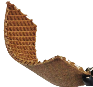
3D-Printed Hygroscopic Wood
