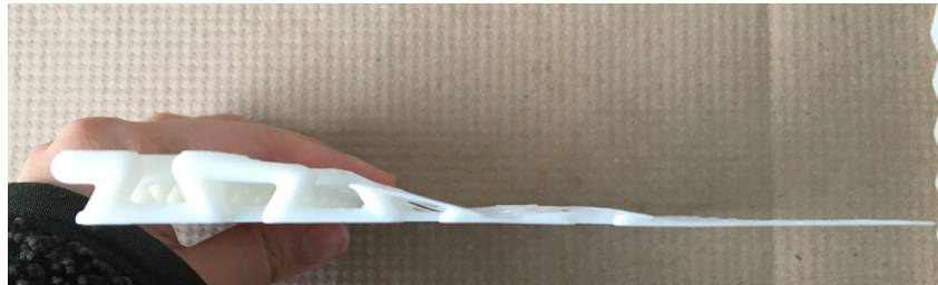
Fig.38 Right: 3D-print failure resulting in 2D to 3D gradation effect Fig.39 Bottom: Iteration diagram of auxetic material functional gradation design
