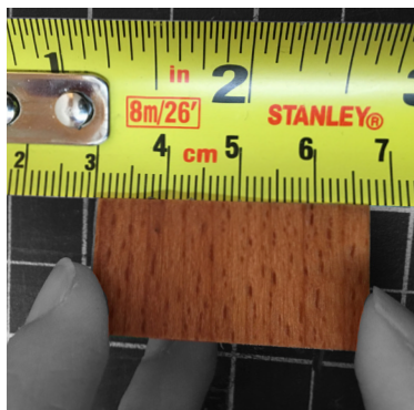
Fig.61 Wood Dry vs Wet Dimension Top: Dry state measuring 33 mm Bottom: Wet state measuring 37mm
