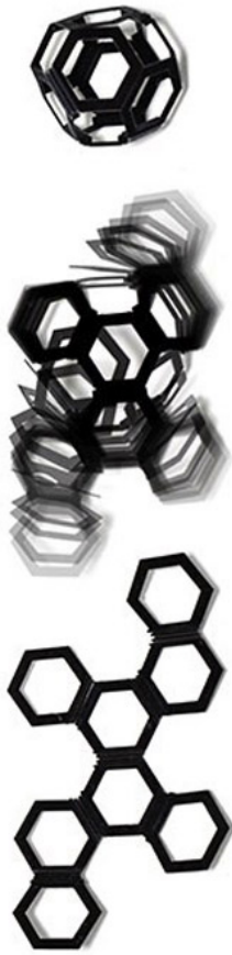
Fig.16 2D shape self-morphing into 3D ball in response to water, 4D Printing: Tuncated Octahedron by Self-Assembly Lab, MIT+ Statasys Ltd+Autodesk Inc.
