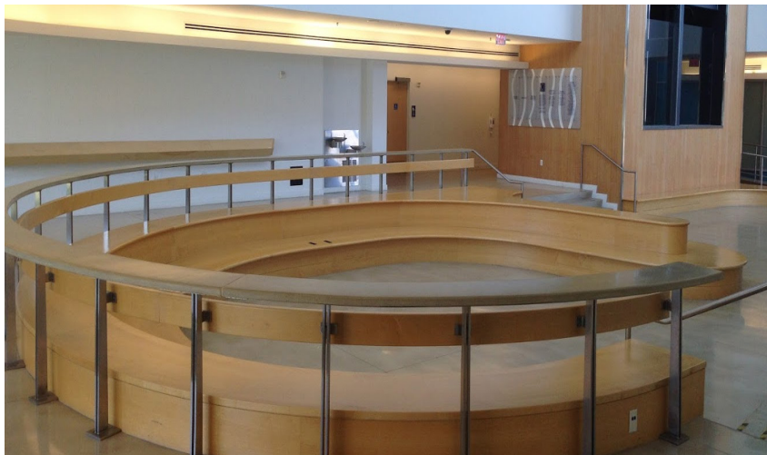
Fig.8 U-shaped podiums designed to allow front row view for every student for easy sign language, The DeafSpace Project by Gallaudet University, 2005
