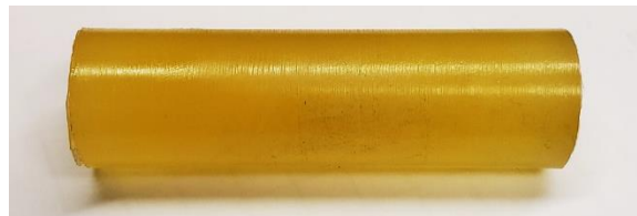
Figure 3.6. A hand-cast neat epoxy cylinder.
