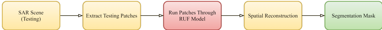
Figure 4.5: Model testing pipeline. Input SAR image is processed as illustrated in Fig. 4.2 to feed patches serially to the trained RUF model for inference. These patches are then reconstructed to yield the segmentation mask for the whole image.
