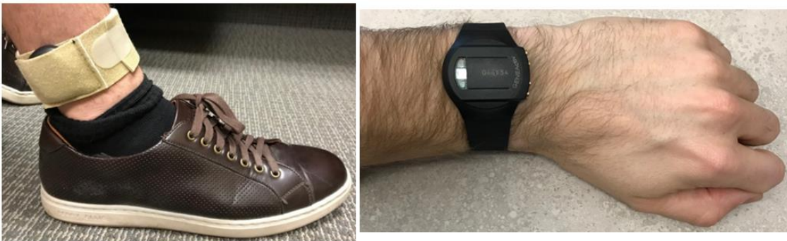
Figure 7: Ankle and wrist GENEActiv accelerometer attachment methods showing the use of custom-made sleeves (left) and original watchband (right).
