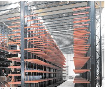
Mecalux Inc Fig. 37. Cantilever racking system of the Interlake Mecalux Inc
