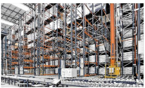
Fig. 45. Vertical lift of the Interlake Mecalux Inc
