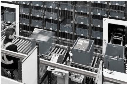
Fig. 49. Packages movement on horizontal carousels (Interlake Mecalux Inc)
