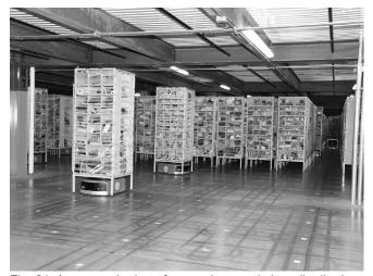
Fig. 21. Automated robots for carrying goods in a distribution facility
