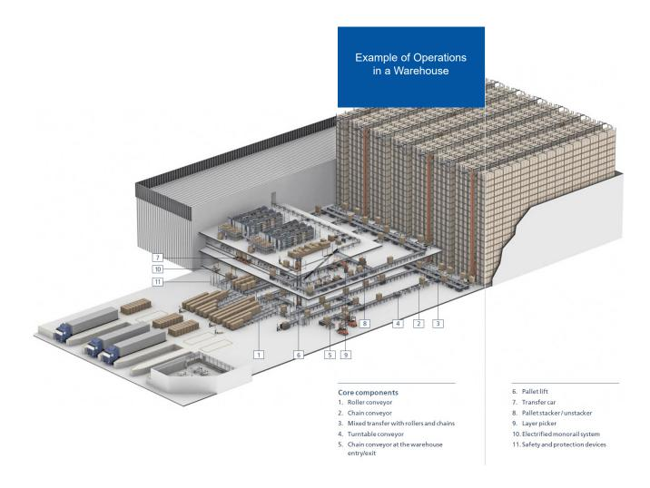
Fig. 30. The example of warehouses operations
