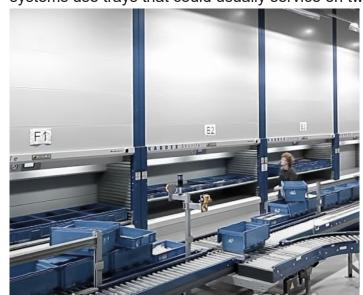
Fig. 41. Sample of vertical lift modules
