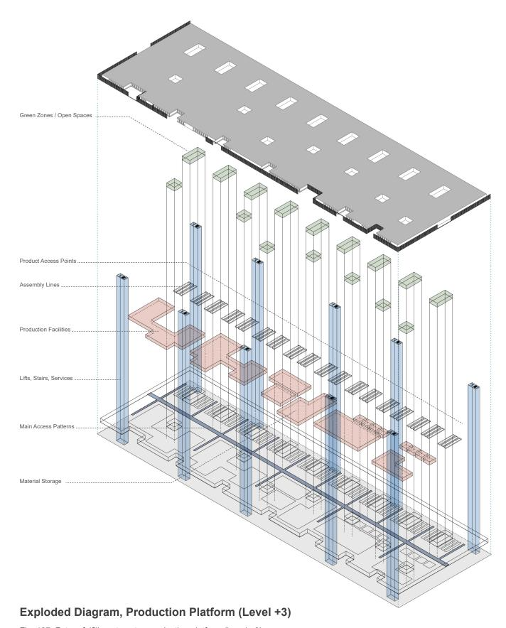
Fig. 137. Future fulfillment center, production platform (Level +3)
