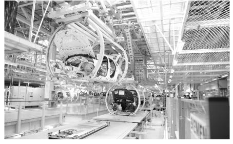
Fig. 103. BMW assembly line, one of the examples of automated, highly mechanized productions systems in which large number of tasks are done by robots and machines.
