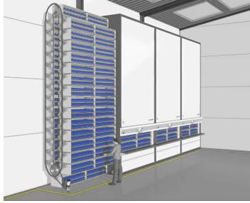
Fig. 51. Structure of vertical carousels
