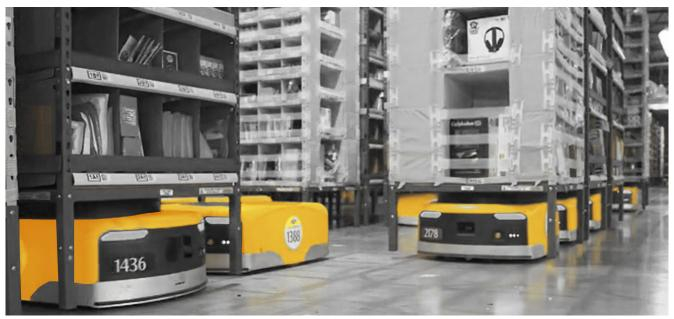
Fig. 106. A robot bringing a shelf for the pickup of items in an Amazon automated fulfillment center
