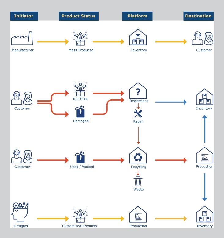
Fig. 116. Fulfillment center material procedures
