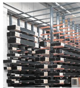
Fig. 34. Cantilever racking system of the Interlake
