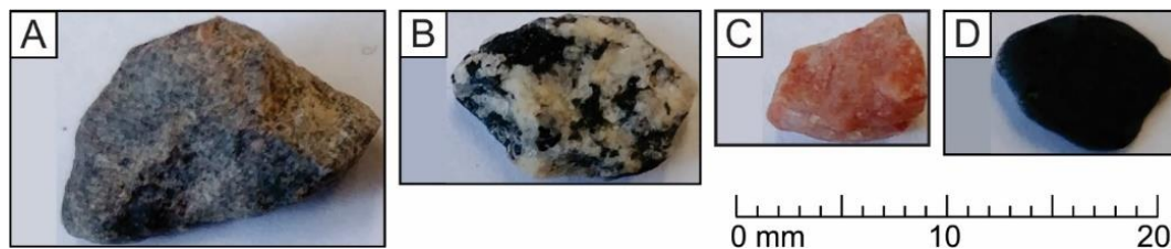
Figure 2-6: Representative grains for clast lithology classification. A) Metasedimentary; B) White Igneous; C) Pink Igneous; and D) Mafic. Clasts have been washed and sorted at the University of Waterloo Quaternary Laboratory.
