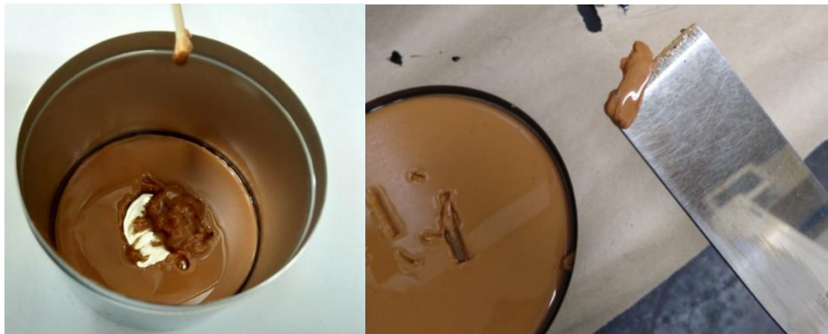
Figure 3- 7 Self-healing elastomer following the second and third attempts using curing Method C
