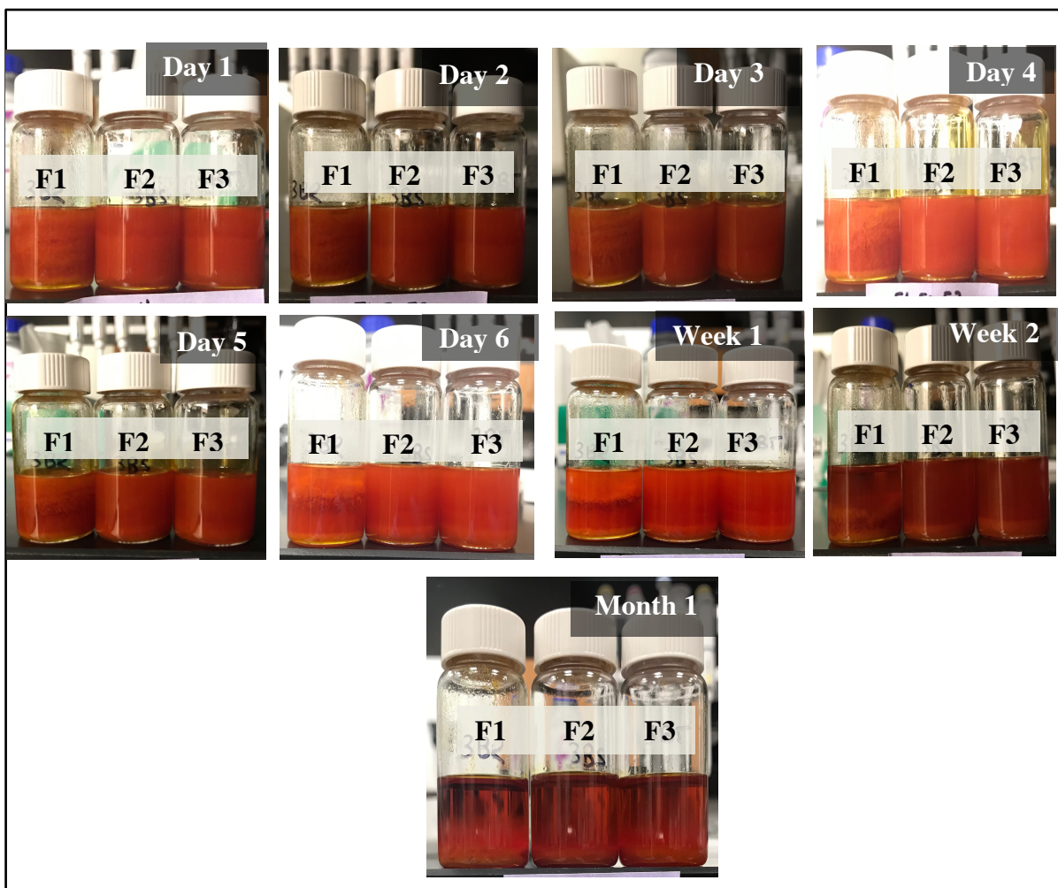
Figure 5-27: Phase separation in microemulsion formulations F1, F2 and F3 after exposure to light over the period of one month.
