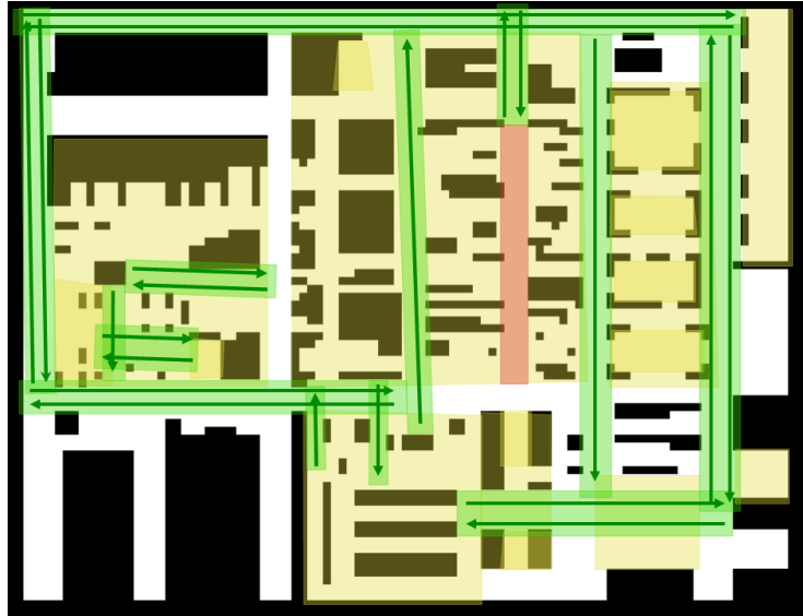
Figure 5.6: Example specification from participant 5. Reduced speed rules are marked in yellow, road rules in green, and avoidance rules in red.
