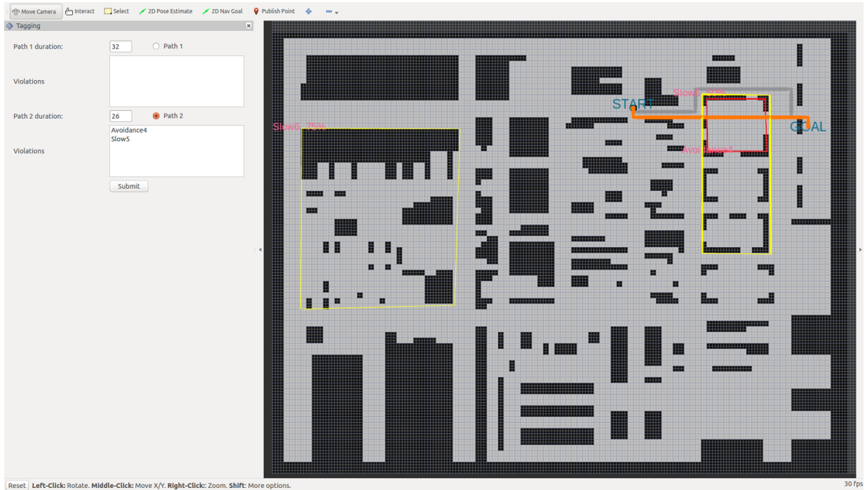
Figure 5.5: Preference learning UI displaying duration and traffic rule violations for each path. Additionally, the violated traffic rules are also highlighted on the map.
