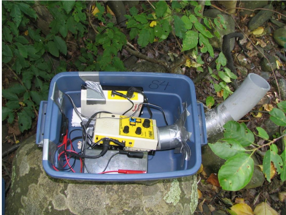
Appendix 2-A. Close up of Anabat II acoustic monitoring system used in sampling during 2005-2006 in southwest Nova Scotia, Canada. Detector with microphone placed in tub with a PVC elbow joint for weatherproofing (photo by Lesley Farrow).
