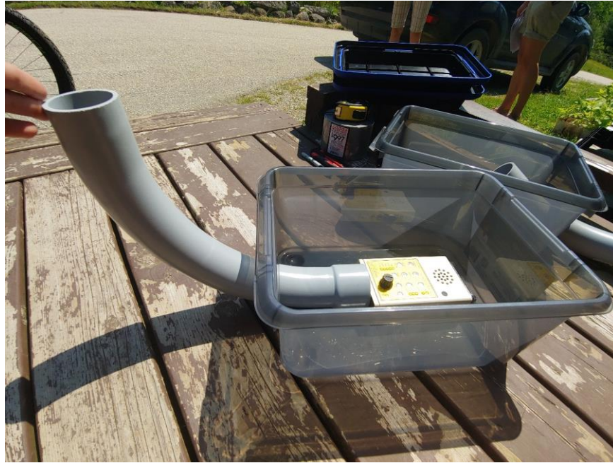
Appendix 2-E. Close up of the replicated Anabat acoustic monitoring setup used during 2005/2006 sampling and acoustic equipment comparison tests with an Anabat SD1. The detector and microphone were placed in tub with a PVC elbow joint for weatherproofing.
