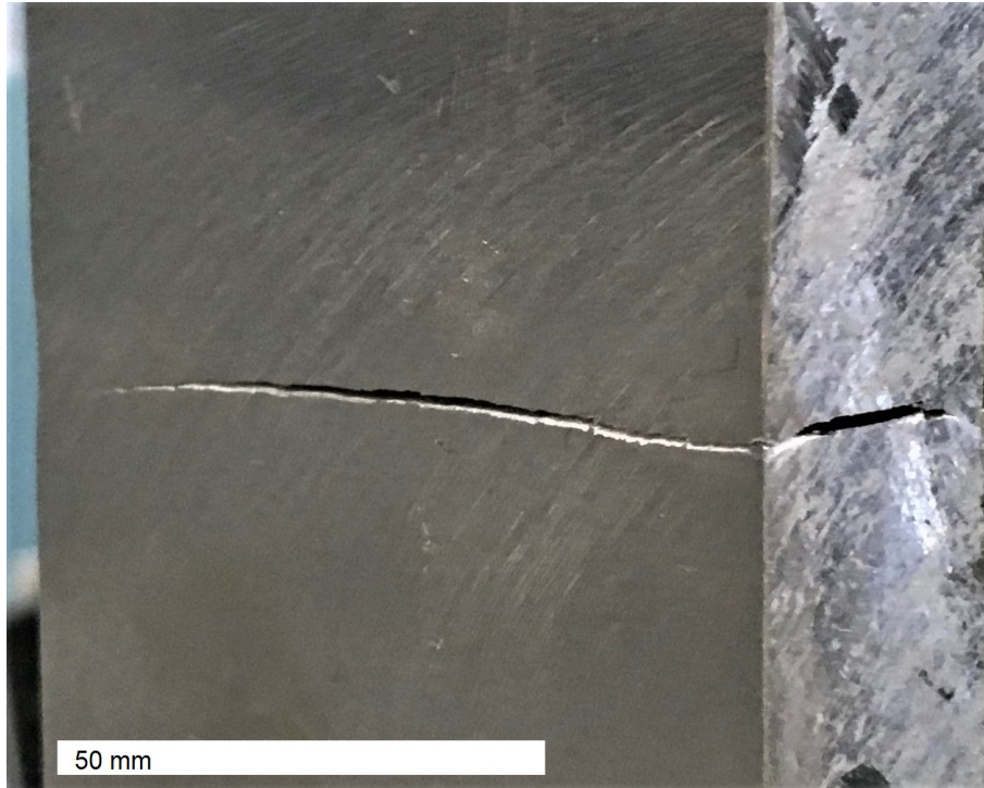
Figure 3.8: A cracked sample just before failure. The weld is difficult to see as its reinforcement was ground off, but the crack grows through it.
