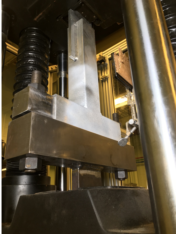
Figure 7.4: A tubular sample ready to be loaded in the MTS 600 kN frame, attached by the stiff steel connector to the grips.
