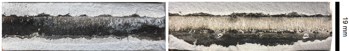
Figure 6.1: On the left, a weld with a penetration specified at 50%. On the right, a weld with 70% specified penetration. The actual degrees of penetration were 55% and 44% respectively.
