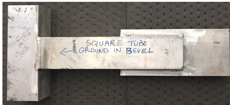
Figure 7.3: Drawing for the tubular samples (top) and typical tested sample (bottom) as part of the flare-bevel weld experimental program. All dimensions are in millimetres.
