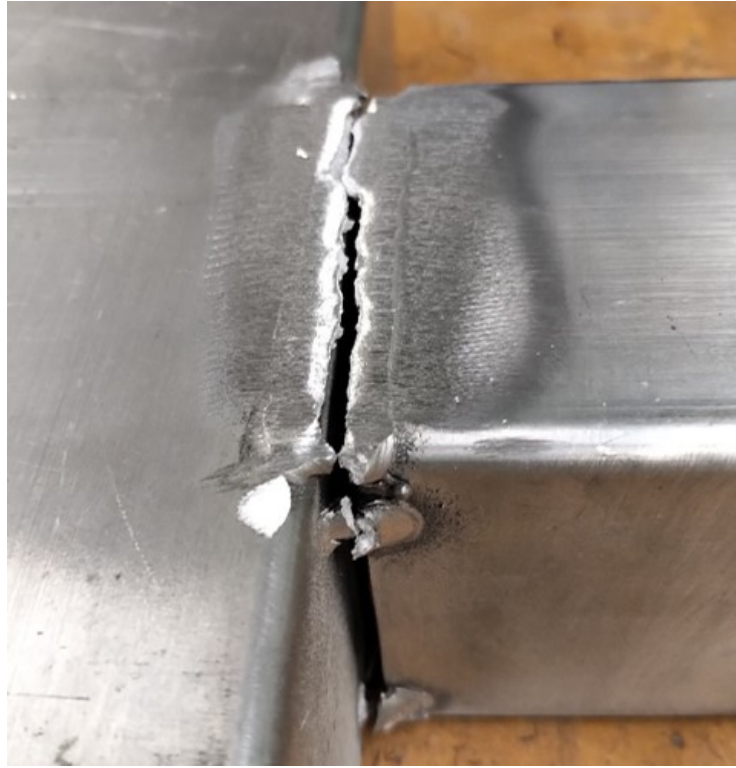
Figure 7.7: A typical failed tubular sample, showing the fracture at the interface of the HAZ and the weld metal. The two tack welds were broken before loading began.
