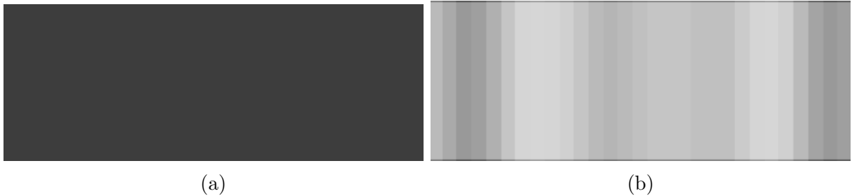
Figure 5.7: Cross-polarization result of IPS cell, (a) Electrodes turned off, (b) Electrodes turned on.
