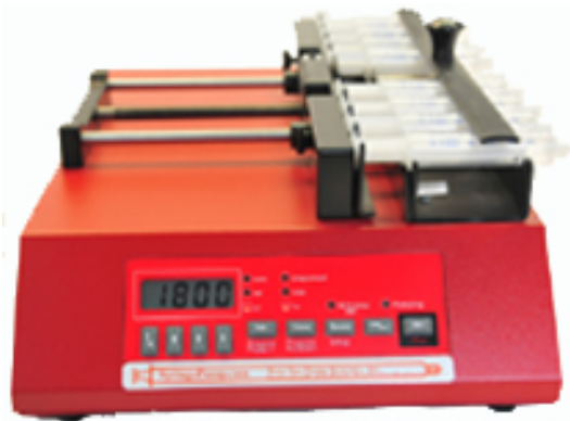
Figure 4.1: Cole-Parmer 75900-50 programmable 6-channel syringe pump
