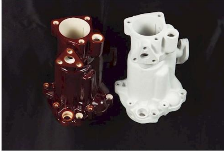
Figure 2-11 Mg oil pump housing with Tagnite coating: Tagnite with paint (left); Tagnite alone (right) [81]
