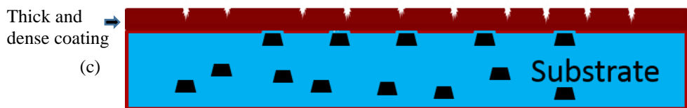
Figure 4-9 Schematic forming procedure of the Mn-P coating obtained by a two-stage conversion coating process: (a) the bare Mg alloy after cleaning pretreatments; (b) after Low pH treatment (LP coating); and (c) after High pH treatment (HP coating).
