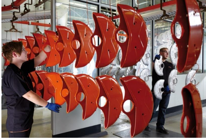
Figure 2-13 Mg engine parts using powder coating which shows perfect appearance and excellent protection [91]
