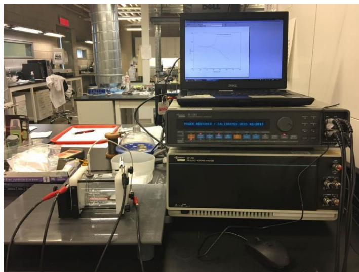
Figure 3-5 The Solartron Analytical 1287A potentiostat/galvanostat and Solartron 1255B frequency response analyzer use for electrochemical testing
