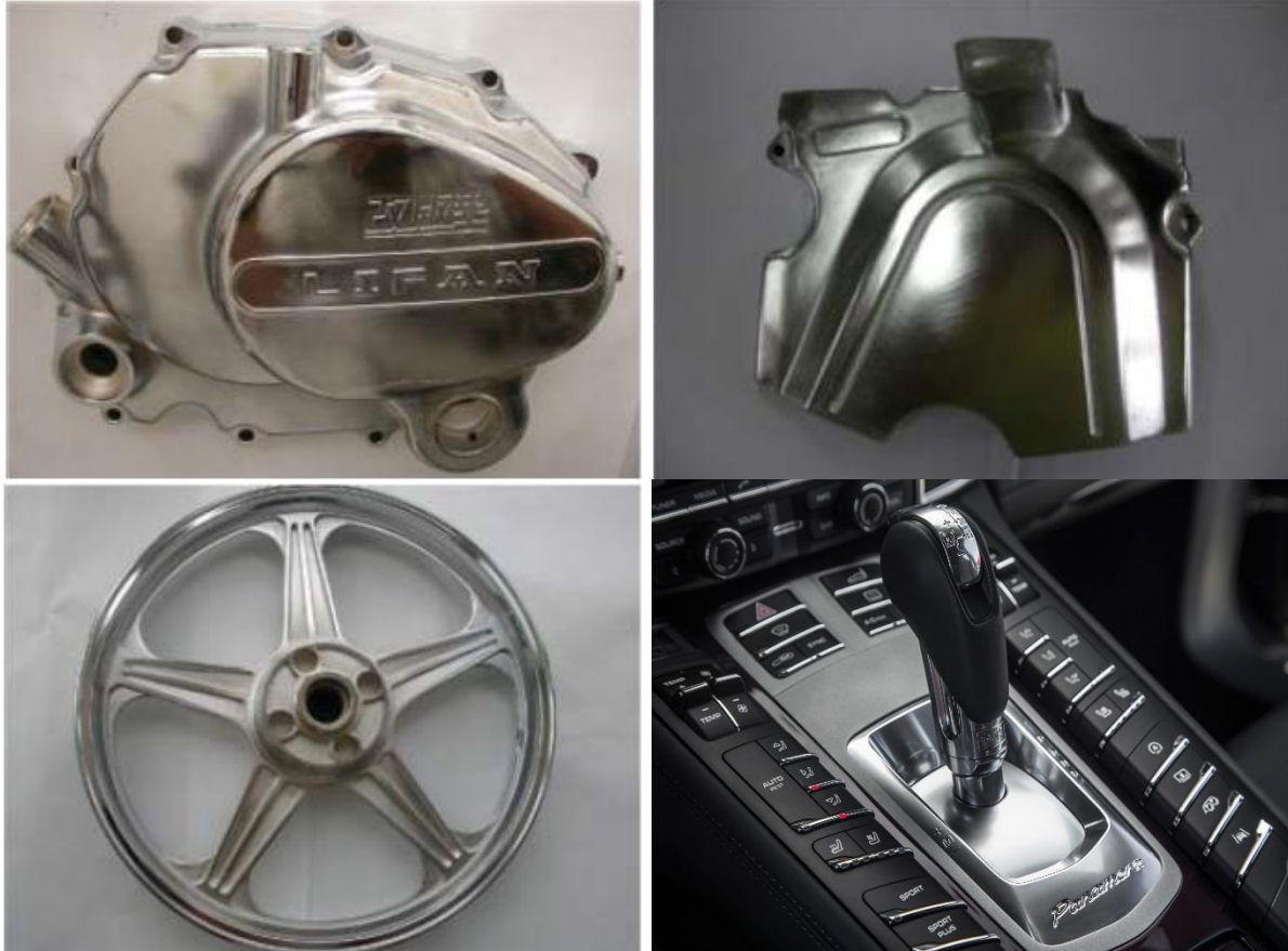
Figure 2-12 Examples of plated Mg components: (a) Top cover of Mg alloy AZ91D engine using direct electroless Ni-P plating followed by Cu/Ni/Cr plating (b) Back cover of Mg alloy AZ91D engine using Zn immersion followed by Cu/Ni/Cr plating (c) Motorcycle wheel hub of Mg alloy AM60 using Zn immersion followed by Ni plating and Cu/Ni/Cr electroplating (d) Interior panel of Porsche Cayenne using Zn immersion followed by Cu/Ni/Cr plating [86]
