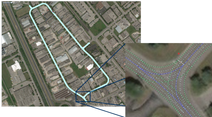
Figure 4.3: A lanelet representation overlaid on a satellite image of a road. Green dots represent the waypoints constituting the right lanelet boundary, while blue and white dots represent the left boundary and centerline respectively.
