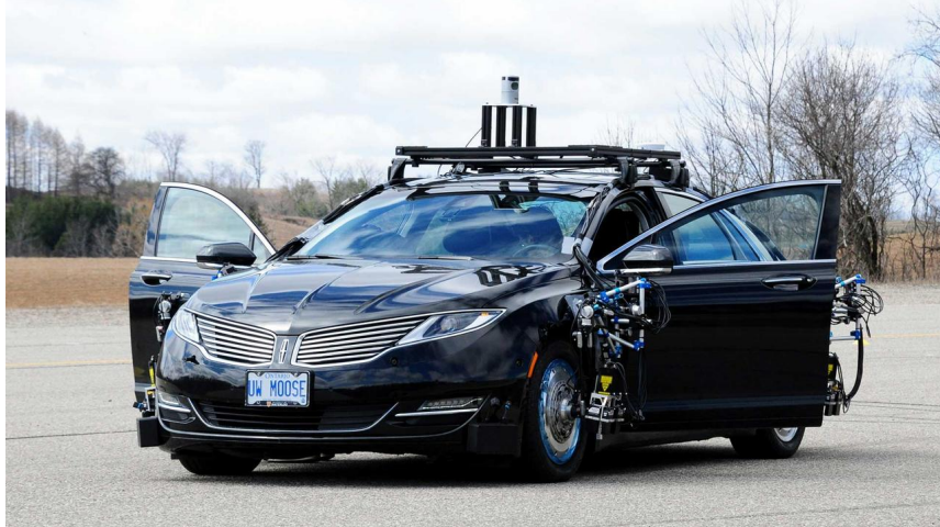
Figure 4.2: The Autonomoose, a 2017 Lincoln MKZ, serving as a platform for autonomous vehicle research at the University of Waterloo.
