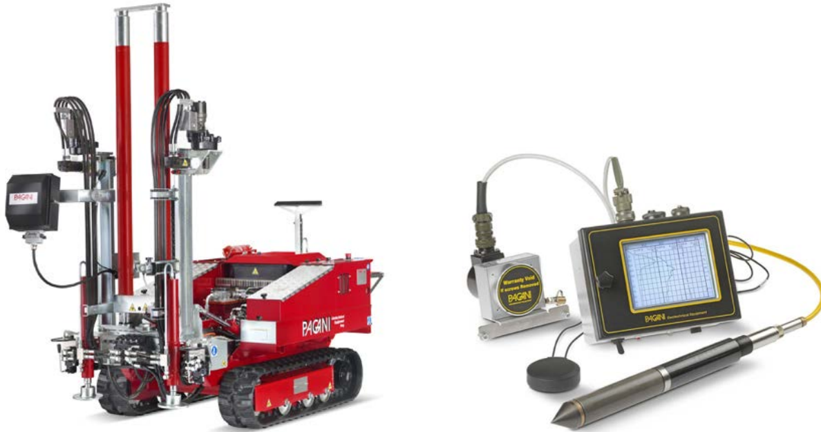
Fig. 6-5: Equipment used for the seismic cone penetration test (sCPTU)
