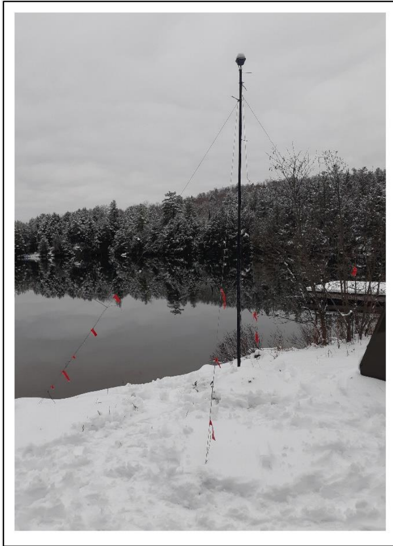
Figure 4 2. GNSS tower installation on the shore of MacDonald Lake on November 19, 2019.
