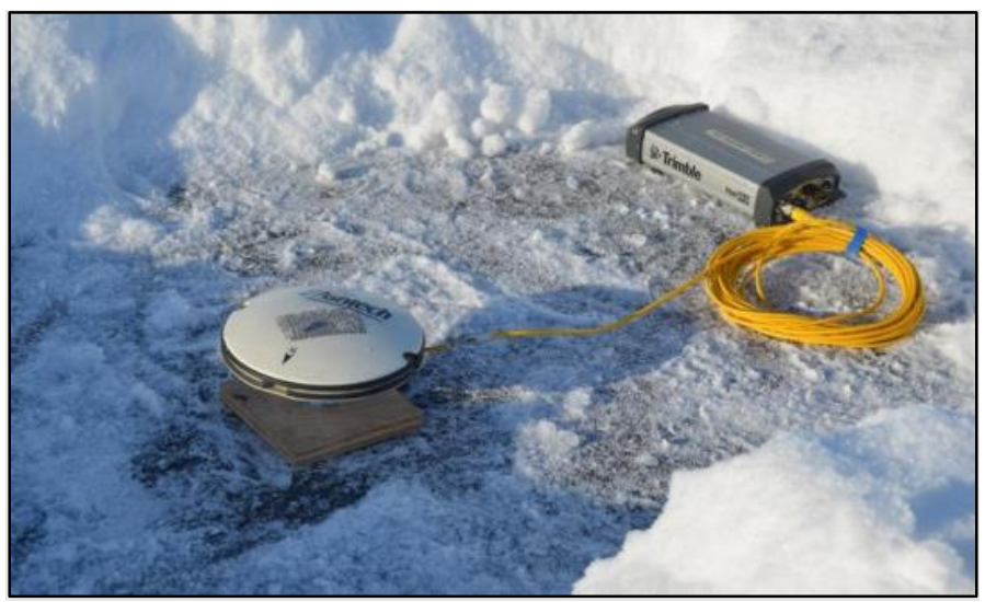
Figure 3.4. GNSS antenna and receiver setup on the lake ice surface.
