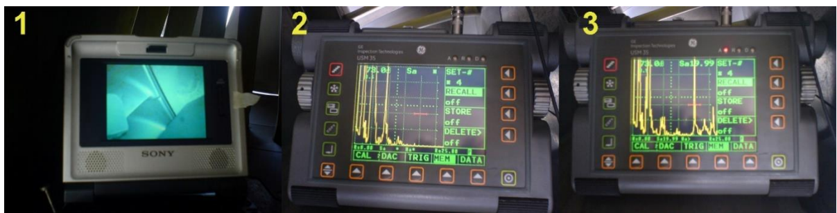
Figure 1-1 Example of ultrasonic test for jet engine turbine blade root test.
