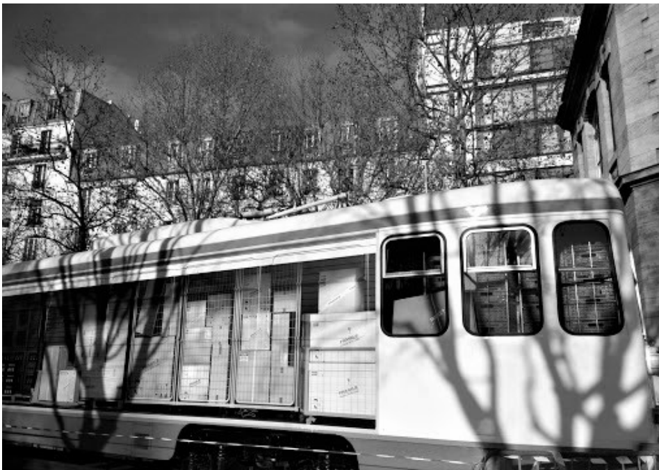
fig. 2.6 TramFret runs adapted freight trams scheduled in between passenger trams
