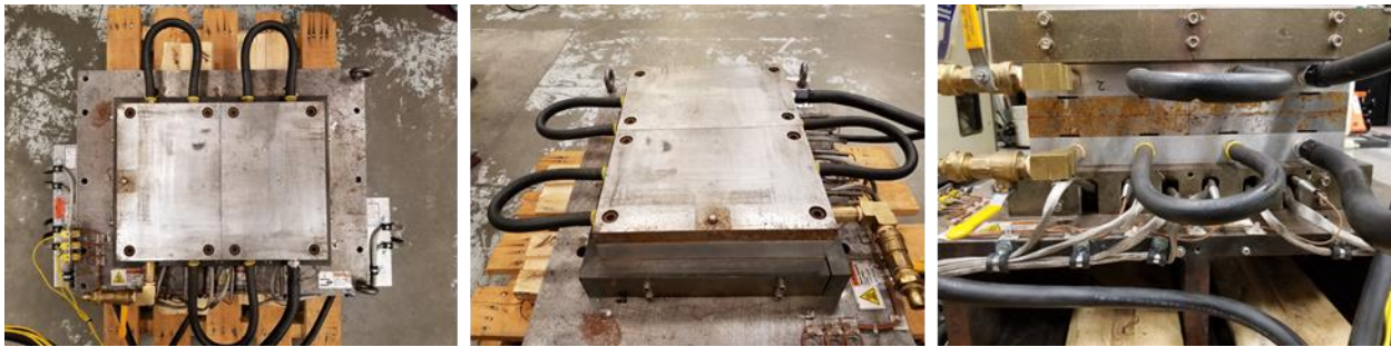
Figure 28: Picture of flat die with cooling channels present
