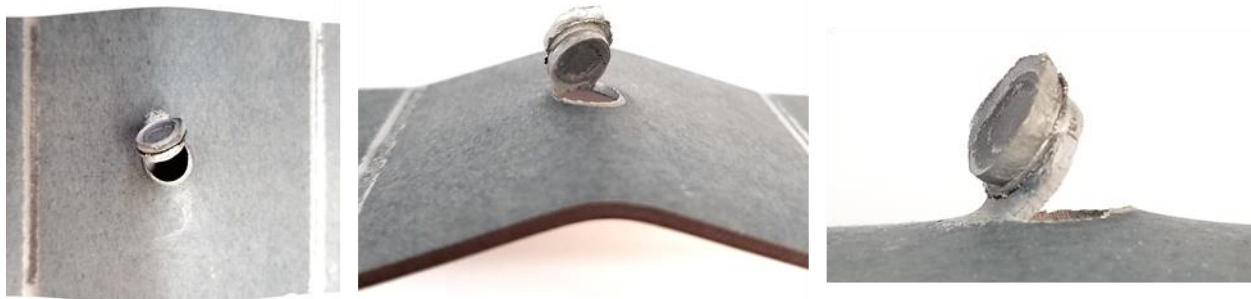
Figure 44: Close up of the Ductibor® 500-AS 1.6 mm cross tension test showing shared asymmetric pull out.
