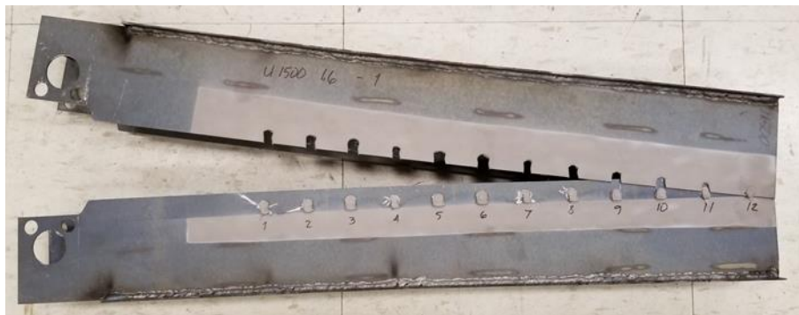
Figure 117: Usibor® 1500-AS 1.6 mm Caiman Mode III quasi-static specimen showing tear out failure.
