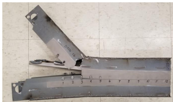
Figure 89: Caiman Mode III Ductibor® 500-AS 1.6 mm quasi-static specimen that buckled.
