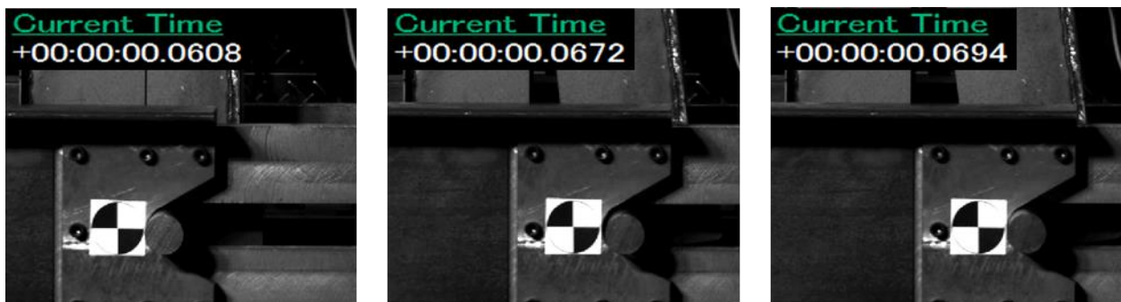
Figure 94: Caiman Mode III dynamic high-speed images of Usibor ® 1500-AS 1.2 mm specimen showing pin and sled contact. Left) Initial contact; Centre) Loss of contact; Right) Secondary contact.
