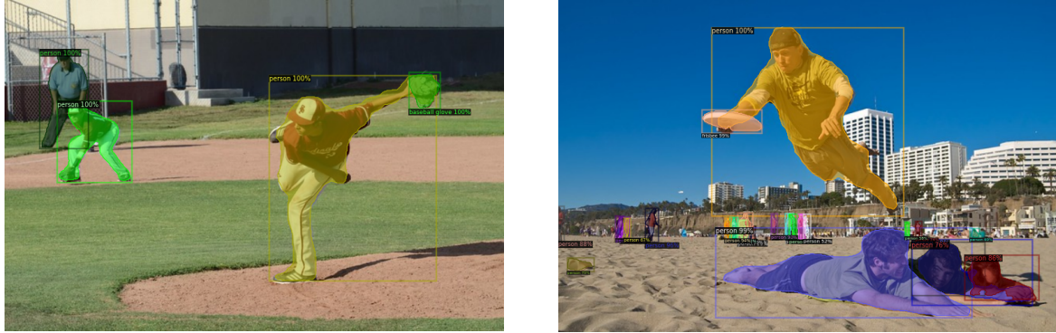
Figure 1.6: Objects in the image on the left have different scales and have the same class (person). Objects in the right image are the same class but different aspect ratios. Images were taken from the COCO dataset [33]
