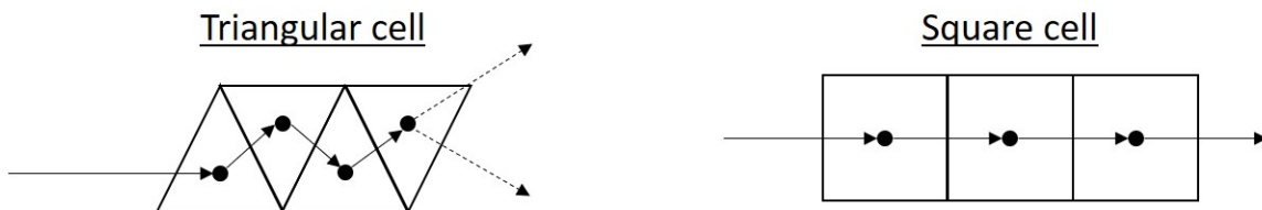
Figure 3.4 Difference in flow estimation between triangular and square cells
