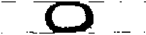
(e) Application of a threshold to retain only dark values (i.e. the droplet shape).
