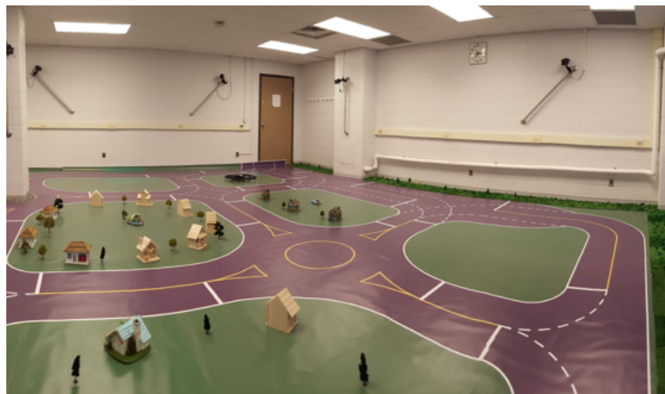
Figure 4.1: Scaled autonomous vehicle test platform developed in SHEVS lab
